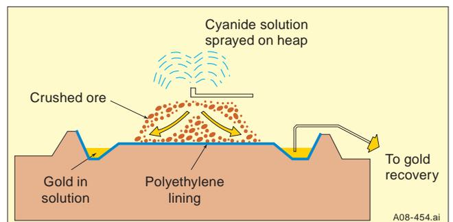
**Figure 7.** Heap leach process at Union Reefs mine (redrawn from 1996 Acacia Resources Annual Report).
