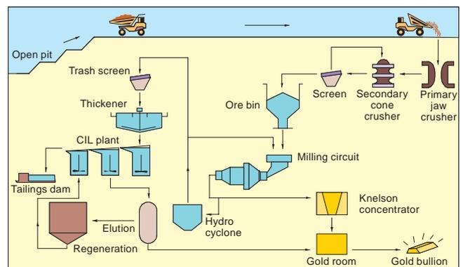
**Figure 6.** Typical Carbon-in-Leach (CIL) plant: gold processing circuit at Union Reefs mine (redrawn from 1996 Acacia Resources Annual Report).
