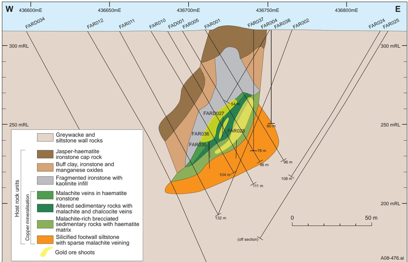
Figure 64. Cross-section of Billy Boy deposit (Giants Reef Mining 1999).
