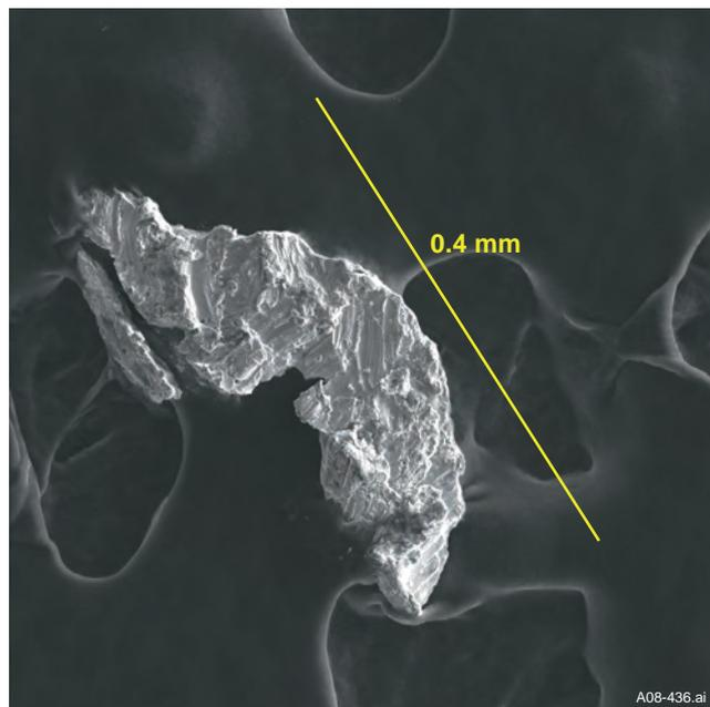
**Figure 19.** SEM image of gold grain from matrix of conglomeratic basal unit of Westmoreland Conglomerate at 0221395mE 8059025mN.
